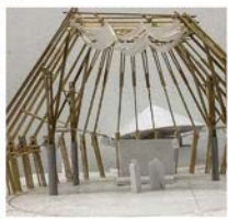
Extremely sustainable: cut and used between 3 and 5 years, stronger than concrete and steel yet highly flexible and lightweight, locally abundant Bamboo - Bamboo Restaurants / Vietnam
